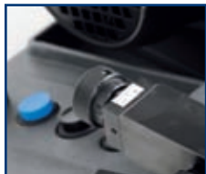
2 Tracer point with micrometric adjustment.
