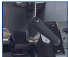
1 2 side jaws which permits: a) duplication of mortice keys b) duplication of front mortice keys.
